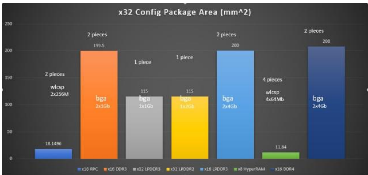
Figure 8. PCB area for memory packages for x32 memory subsystem (click on image for larger view).
